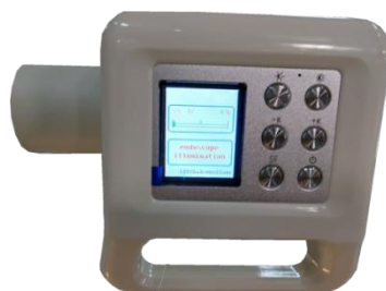
LCD screen panel with endoscopy function
